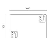
Top and Base- In lacquered wood Vertical Posts- Cladded in eco leather Hanging Rails- In metal and eco leather
